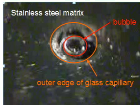
Figure 9. Frame of a video showing a gas bubble emerging only from the glass capillary
