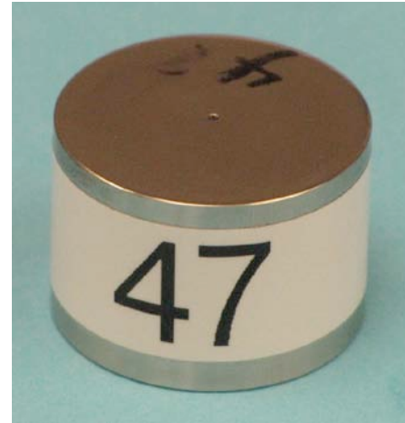
Figure 8. Capillary-based permeability standard (47 micron diameter channel).
